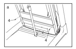
Lower the treadmill (see HOW TO LOWER THE TREADMILL FOR USE on page 30). Remove the four indicated #8 x 3/4" Screws (4), and remove the Motor Hood (44).
